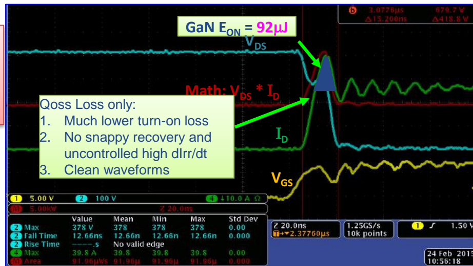
Half bridge turn-on 400V/20A – GaN E-HEMT
