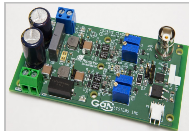
100V GaN E-HEMT Full Bridge Evaluation Board, optimized for Class D Amplifiers
