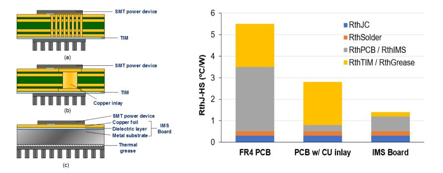
The thermal performance is enhanced compared with the PCB solution.
