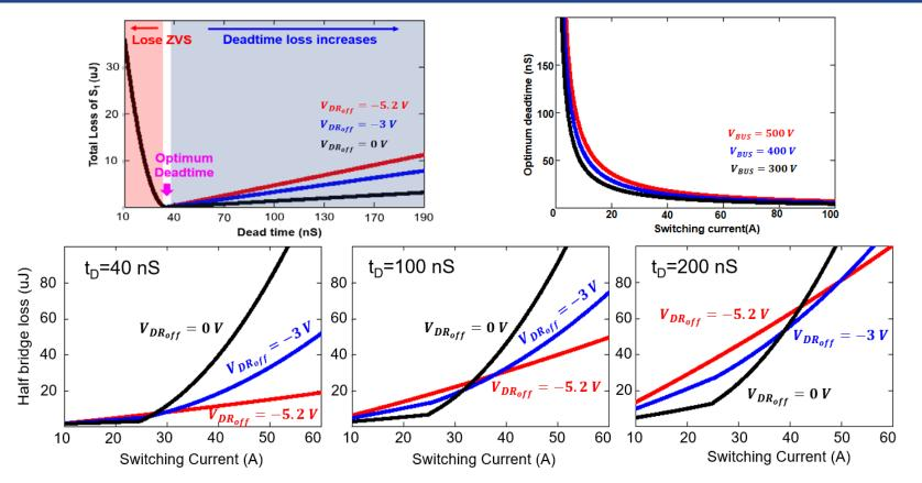
Half-bridge overall loss vs. switching current under different negative turn-off gate voltage  $V_{DRoff}$  (a) with deadtime  $t_D$ =40 nS, (b) with deadtime  $t_D$ =100 nS, (c) with deadtime  $t_D$ =200 nS.
