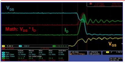
Hard switching turn-on of a GaN E-HEMT @ 400V/22A
