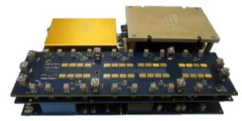
7 kW Level-2 EV onboard charger from Hella (soft-switching)
