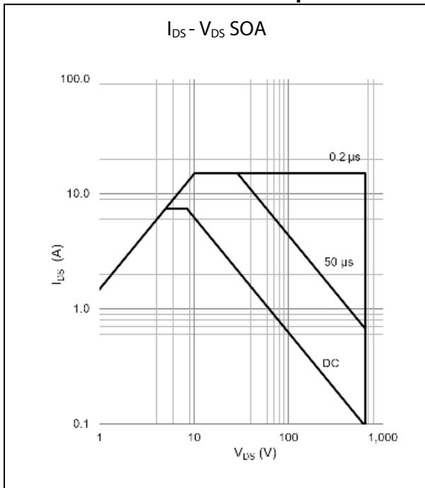
Figure 13: Safe Operating Area @  $T_{case} = 25^\circ C$
